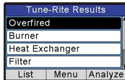
display a prioritized list of most likely potential issues to investigate. A drill-down into a "checklist" helps to keep track and record what has been inspected, adjusted, repaired or found to be an issue.
