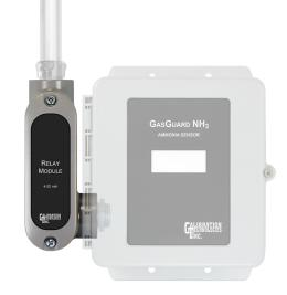
ANALOG INPUT IMPEDENCE: 10 Ohms RELAY: (1) SPDT relay, Form C contacts, 8A @ 24VDC, 8A @ 120VAC, normally energized, non-latching, Status LED shows relay state RELAY TIME DELAY: 2 second on, 10 seconds off FAIL SAFE FUNCTION: Sensor fault (0.5 mA) or loss of power will de-energize the relay FAULT SETPOINT: 1 mA ALARM DIRECTION: Upscale only ENCLOSURE: Powder coated aluminum, LR conduit body OPERATING TEMPERATURE: -40°F to +122°F OPERATING HUMIDITY: 0-100% RH, condensing WARRANTY: 2 years
