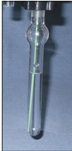
Figure 8.1-4: Look for Bubbles in the sparge bottle.
