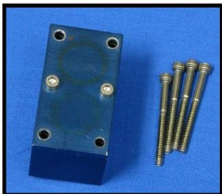
Figure 7.3-2: Four corner screws removed and scrubber removed from FROG
