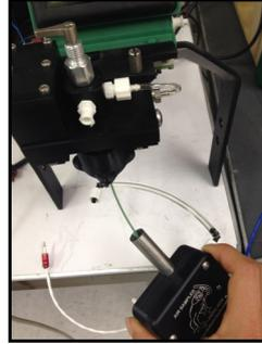
2. Connect the air sampler's valve connector to the FROG valve connection. This connection supplies power to the air sampler.
