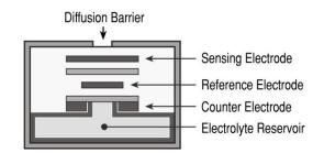
Figure 1 Construction of Electrochemical Toxic Sensor
