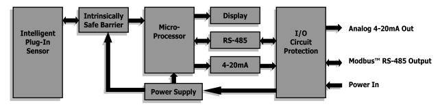
Figure 3 ITM Circuit Functional Block Diagram
