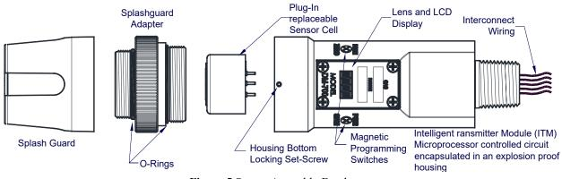
Figure 5 Sensor Assembly Breakaway
