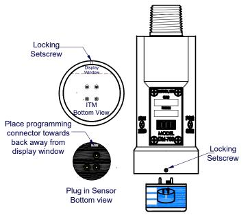
Figure 19 Sensor Cell and ITM Mating
