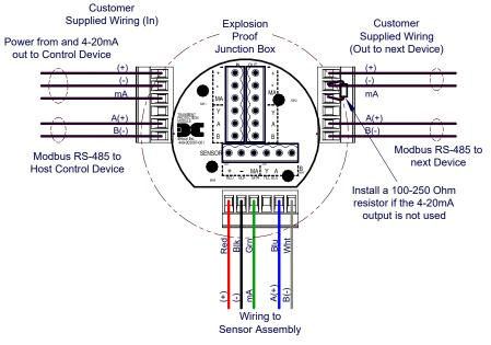
Figure 13 Sensor Wire Connections
