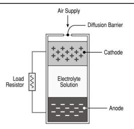
Figure 2 Construction of Galvanic Cell
