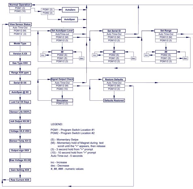
Figure 16 DM-700 Software Flowchart
