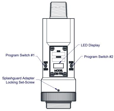
Figure 4 Sensor Assembly Front View
