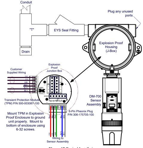
Figure 12 Typical Installation
