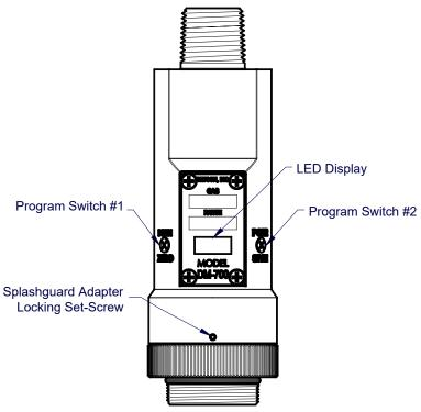
Figure 15 Magnetic Programming Switches
