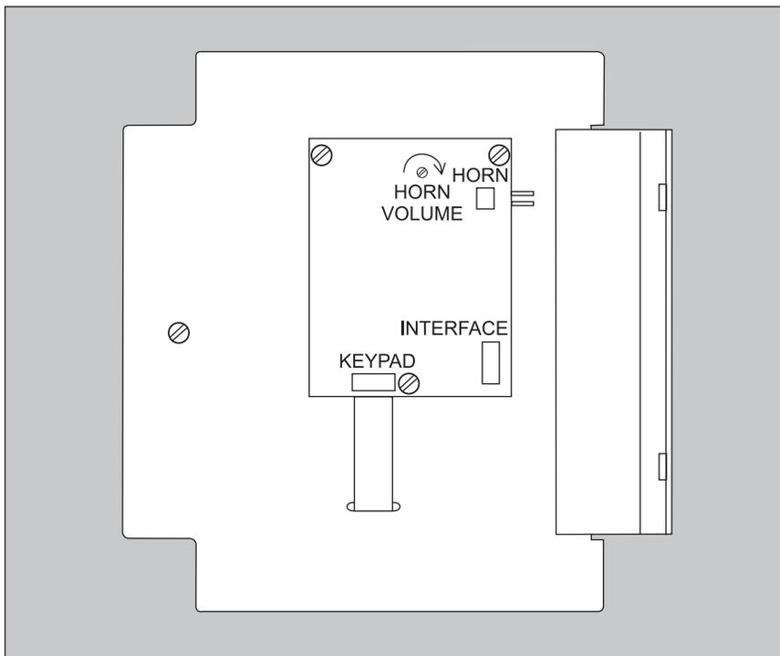
*Figure 5: Adjusting the horn volume*
