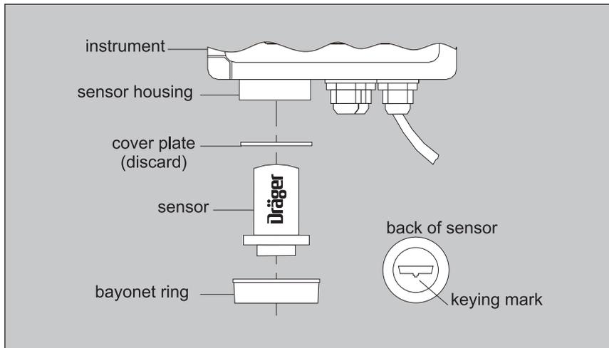
Figure 4: Installing the sensor
