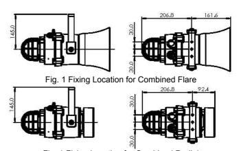
Fig. 1 Fixing Location for Combined Radial
