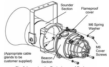
Fig. 2 Accessing the Explosion proof Enclosure.
