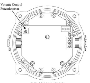
BExCS110-05D DC Fig. 9 Location of Volume Control Potentiometer
