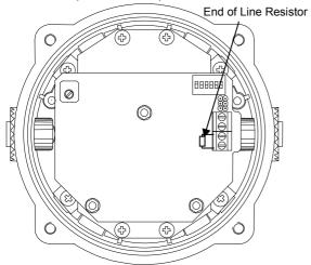
Fig. 8 End of Line Resistor Placement
