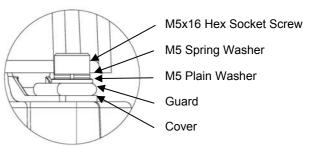
Fig. 13 Cover and Guard Fixtures
