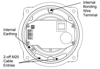
Fig. 3 Internal View of Cover
