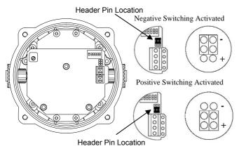
Fig. 7 Stage Switching Polarity
