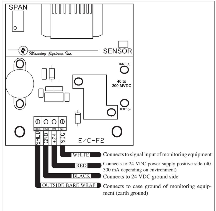
**Figure 2: Wiring diagram for the EC-F2 Sensor**
