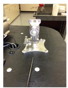
The next step in the process is to attach the mounting brackets (pn: 888270) to whatever surface according to the specifications of the project. Please note the orientation of the detector mount so that the mounting brackets are pointed in the correct direction.
