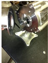
It is now time to attach the alignment telescope to perform the fine alignment. However, you must first remove the protective visor from the front of the detector or flash source.
