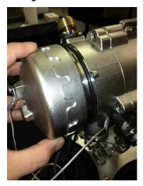
Now that the detector and flash source have been attached to the mounting brackets it is time to connect power and signal wires to the appropriate terminals. But first you must remove the back cover from the unit. Simply screw the unit off counter-clockwise revealing the wiring terminals.
