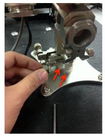
Now it is time to loosen both tensioning bolts on both the vertical and horizontal alignment shafts. This will allow the unit to have free range of motion using your hands to perform the rough alignment. Please note that when doing vertical adjustment it is important to hold the unit so it does not swing down with force.
