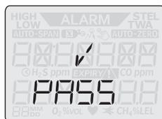
3. When the zeroing process is successfully completed, *PASS* appears.
