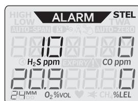
As a permissible exposure limit, a short-term exposure limit (STEL) is the acceptable average exposure over a short period of time as long as the TWA is not exceeded. The default duration is 15 minutes.
