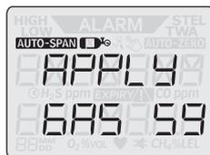
5. When **APPLY GAS** appears with a 60-second countdown, apply the calibration gas to the detector at a flow rate of 250 to 500 ml/min before the countdown is completed.
