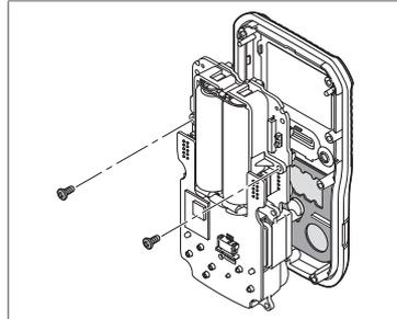
2. Loosen the two screws on the PCB to remove it from the front panel.
