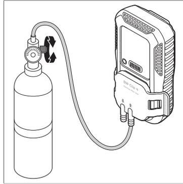
3. When *APPLY GAS* appears on the display of the detector, open the cylinder valve by turning the pressure regulator knob counterclockwise.
