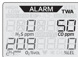
As a permissible exposure limit, a time-weighted average (TWA) is the acceptable average exposure over a specified period of time. The default period is 8 hours.
