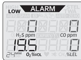
When a gas alarm occurs, the gas detector starts beeping, flashing and vibrating simultaneously and continues until the alarm condition is cleared. In addition, the display backlight turns on and the identifier for the responsible gas starts flashing.
