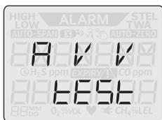
3. *AVVV EEEE* appears as the detector beeps, flashes and vibrates to test the function of audible, visual and vibrating alarms. When *EO PASS HOLD* appears, press and hold the button for 1 second to acknowledge the test. To fail this test, briefly press the button.
