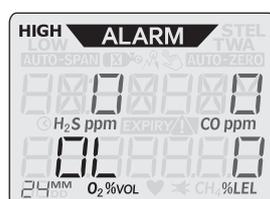
When a gas concentration is over the upper limit of the detection range, an over-limit (OOL) alarm is generated.
