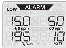
To see low alarm thresholds, get into the *INFO HOLD* menu. Skip ahead until the alarm symbol **ALARM** appears with **TWA**. Press the button again to see STEL, low and high alarm thresholds.
