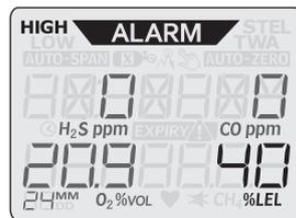
For high, STEL, and out-of-range alarms, the detector generates faster beeps, flashes and vibrations than for the other alarms, to draw more attention.
