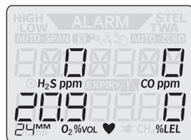
Activate the gas detector in a place where the air is clean and free of hazardous gases. In normal air, the concentration of oxygen is 20.9%.
