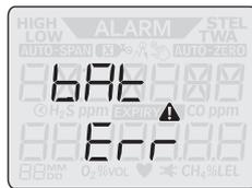
BW Clip4 is designed to run for 2 years without having to be charged. Within 2 years operating time, battery could be discharged depending on the actual use case. BW Clip4 display will show the alarm *bAt Err* and BW Clip4 will be turned off automatically 10 minutes later. Please contact Honeywell Analytics or your distributor for technical assistance.
