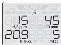
Peak readings are the highest detected concentrations since the last reset. To see the peak readings, choose *I NFO HOLD* from the menu. The peak readings are displayed with the peak symbol
