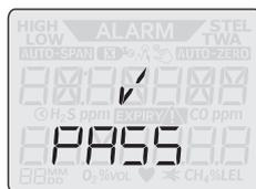
7. When the bump test is successfully completed, *PASS* appears. If it fails, *FAIL* appears with the flashing non-compliance symbol
