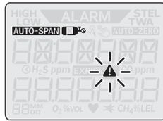
The calibration symbol **AUTO-SPAN** and cylinder symbol
