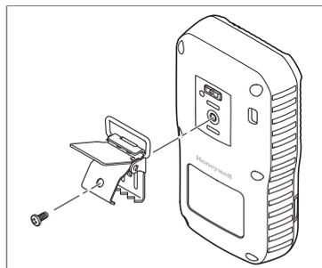
If the belt clip is damaged or loose, replace it with a new one. Insert a screwdriver through the hole in the clamp and loosen the screw to detach the clip. Put a new clip in place and fasten it.
