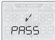
3. When the zeroing process is successfully completed, **PASS** appears. If it fails, **FAIL** appears with the flashing non-compliance symbol
