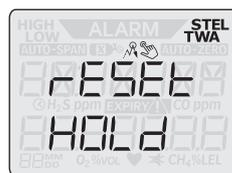
To reset peak, TWA and STEL readings, get into the *I NFO HOLD* menu. Skip ahead until *RESET HOLD* appears with
