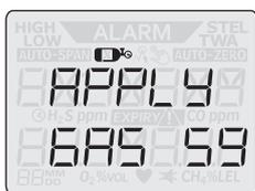
4. When *APPLY 60S* appears with a 60-second countdown, apply the calibration gas to the detector at a flow rate of 250 to 500 ml/min before the countdown is completed.
