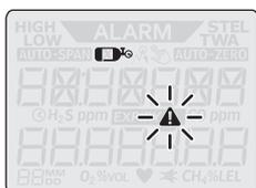
The cylinder symbol
