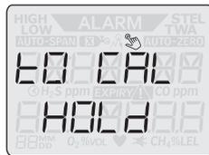
1. Press the button twice in succession to get into the menu, skip ahead to **HOLD CAL HOLD** by repeatedly pressing the button, and then press and hold the button to initiate a calibration.
