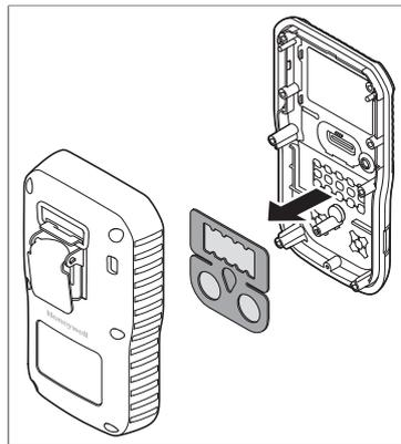
3. Remove the sensor filter from the inside of the front panel.
