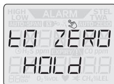
1. Press the button twice in succession to get into the menu, skip ahead to *EO ZERO HOLD* by repeatedly pressing the button, and then press and hold the button to initiate a zeroing process.
