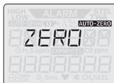
2. *ZERO* appears with the flashing zeroing symbol **AUTO-ZERO**. Wait until this zeroing process is completed.
