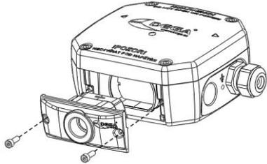
In case of need to replace the sensor module with a new piece, unscrew and remove the cover. Disconnect the sensor module cable from the PCB (1), loosen the sink screw (2) and unscrew the steel cylinder with the sensor (3). Screw the new sensor module, retain it with the sink screw and connect the cable to the PCB. Finally, mount the cover and connect to the power supply.
