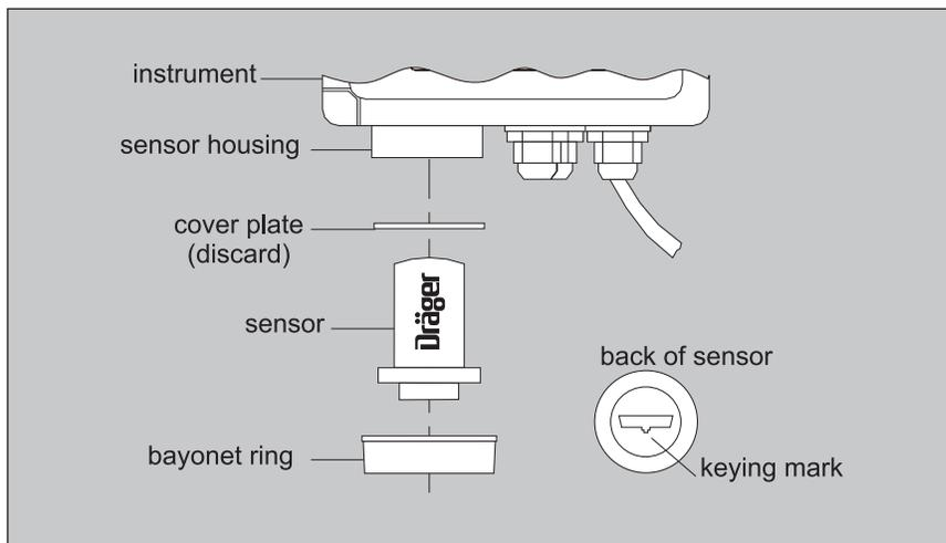
Figure 4: Installing the sensor
