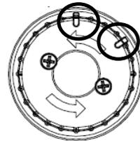
Note: use alignment marks circled to indicate the push button's status /position.
