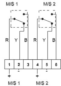
**Unit in 'Operated condition' (button pushed in)**
