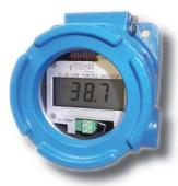
The GDS-54 Loop-Powered Indicator displays 4-20mA variables in their correct engineering units. The GDS-54 has a single 3-1/2 digit LCD readouts with optional trailing "0" for readings up to 19990. Decimal points are DIP-switch selectable. Non-interacting ZERO and SPAN potentiometers allow precise display in any desired engineering unit value.
