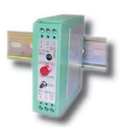
The GDS-54 Loop-Powered Alarm is designed to initiate actions, such as turn on a horn, motor or indicator light when the monitored loop current rises above or falls below a fixed setpoint. It may be installed in any 4-20mA current loop where a fail safe, completely isolated SPDT dry contact relay is needed for switching AC or DC loads.
