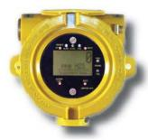
The GDS-56 Loop-Powered Indicator displays loop variables in their correct engineering units, as 30-minute trends and bargraphs. Two trailing dummy "0" characters allow readings up to 999900. All configuration is done using magnetic wands; there are no analog potentiometers or DIP switches to adjust. An optional totalizer function displays up to 10-digit values.
