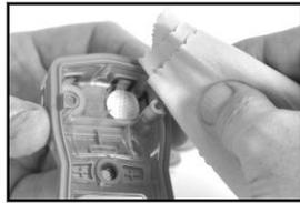
Using a clean, soft cloth, press gently around the filter edge; hold for five seconds to activate the adhesive.
