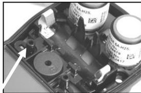
The instrument's interior power button is located below the battery cradle and to the left of the speaker (see arrow above).
