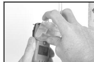
To remove the calibration cup, lift up from the cup's tabs. Set aside or store for future use.
