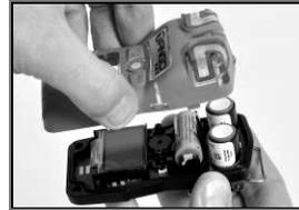
Continue to lift the case top straight up to remove it and to avoid unintentionally loosening the sensors.
