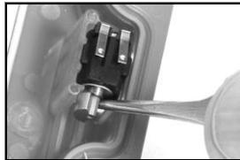
Insert the tweezers between the case top and the motor.
