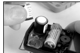
Lift the sensor to remove it.
