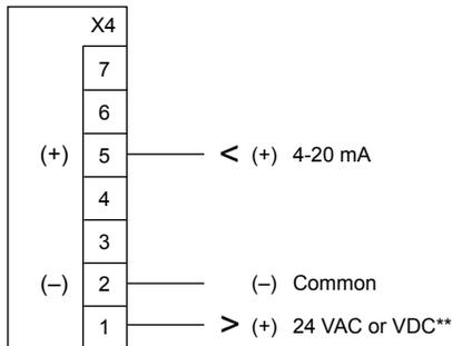
4-20 mA, 2-wire loop-powered sensor/transmitter
