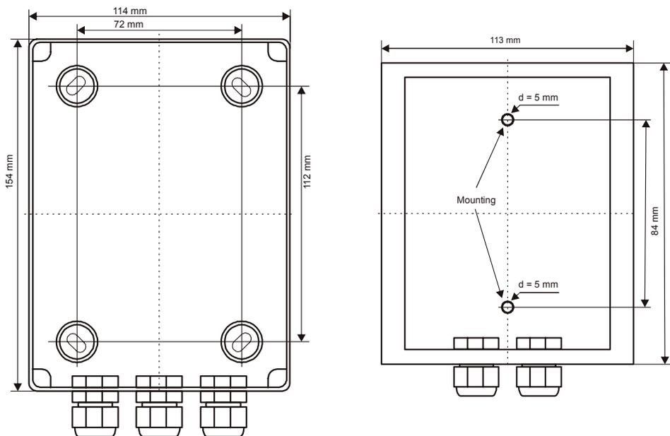
Fig. 01 Standard plastic housing
