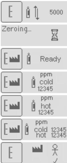
\* Fill an empty (uncontaminated) sample bag with 5000 ppm Helium gas before starting the calibration procedure. Also remove the outer grey probe from the GasCheck G.
