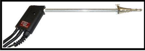
Standard probe: 10" insertion; 9' rugged, braided sheathed sampling line with K-Type t/c (1,200°F max) and silicone hose for combustion applications
