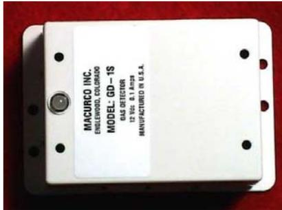
The GD-1S is an all electronic detector of the types of gases that are hazardous in boats, motor homes, and alternately fueled vehicles. The GD-1S operates on 12VDC and is housed in a small plastic case that can mount to a flat surface or over a single gang electric box.
