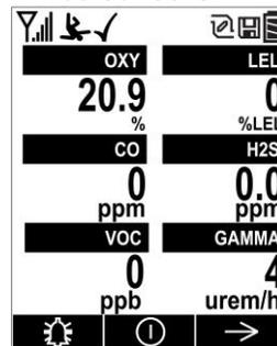
Six-sensor configuration with CO+H<sub>2</sub>S combo sensor.
