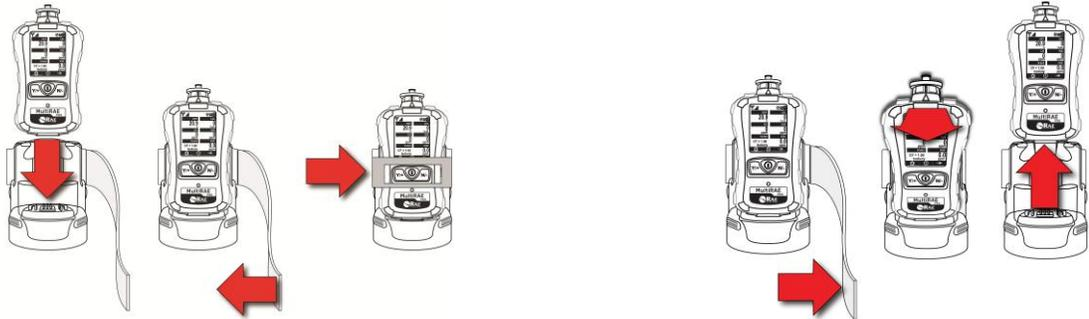
**To secure:** Press the MultiRAE into the cradle and fasten the Velcro strip.
