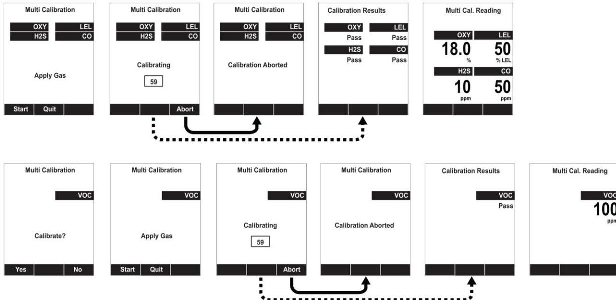
For a multi-sensor span calibration, a constant-flow regulator producing 0.5 to 1 liters per minute should be used, and the calibration cap must be installed on the instrument. Testing and calibration with an AutoRAE 2 must be performed using demand-flow regulators. A calibration cap must not be used. Teflon tubing must be used to test or calibrate the PID sensor. Follow the steps described here to perform a multi-sensor span calibration:
