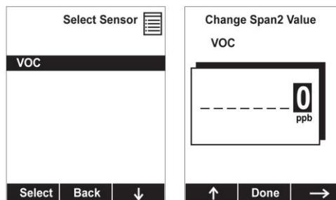
**Note:** Three-point calibration is disabled by default, but can be enabled on MultiRAE and MultiRAE Pro instruments with 10.6eV PID sensors, including high-range ppm and ppb PID sensors. The MultiRAE Lite PID sensor only supports 2-point calibration.
