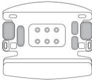
**1. Check bottom of MultiRAE Travel Charger's alignment pins for correct orientation with the MultiRAE.**
