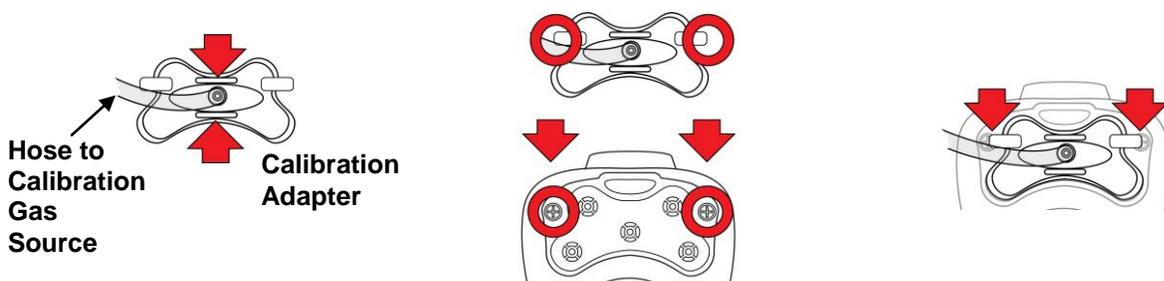
Grasp the small handles on the Calibration Adapter.
