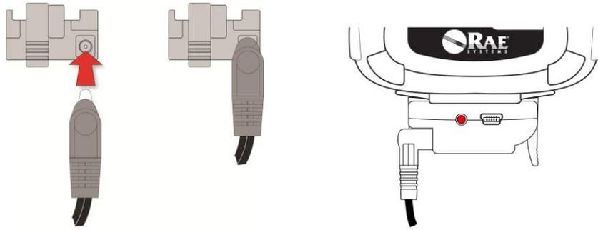
Plug the other end of the charger into a power source (AC outlet or 12VDC mobile power port, depending on the model). When power is applied and the MultiRAE's battery is charging, the LED glows red. The LED glows green when the battery is fully charged.
