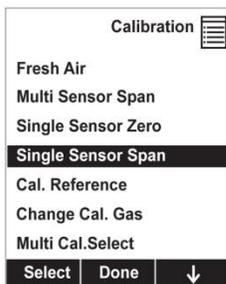
6. Press [Y/+] to start calibrating or wait for calibration to start automatically.
