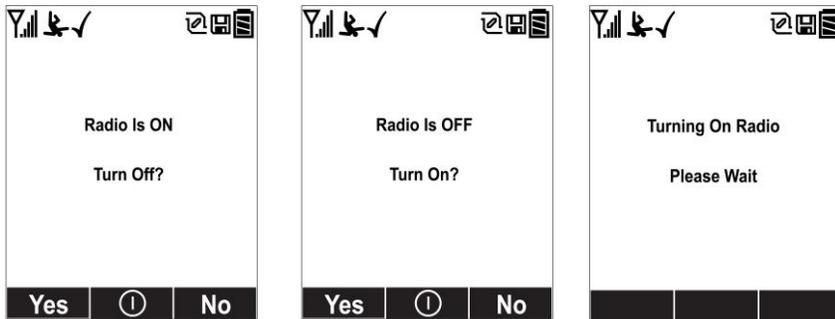
At the Wireless screen, you can check communication with other wireless devices and get other useful information about the wireless settings. The Wireless menu is divided into a sequence of four “pages,” each presenting different information. As you press [Y/+] on each of the “pages,” you advance to the next one.
