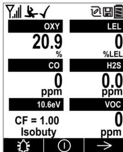
As the MultiRAE is tilted, the gravity sensor detects its orientation and inverts the screen when it is past its horizontal position.
