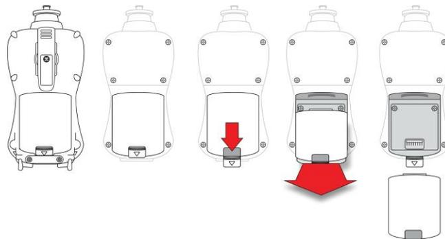
2. Tilt a fully charged battery (or alkaline battery adapter) into the battery compartment and place it in the instrument.
