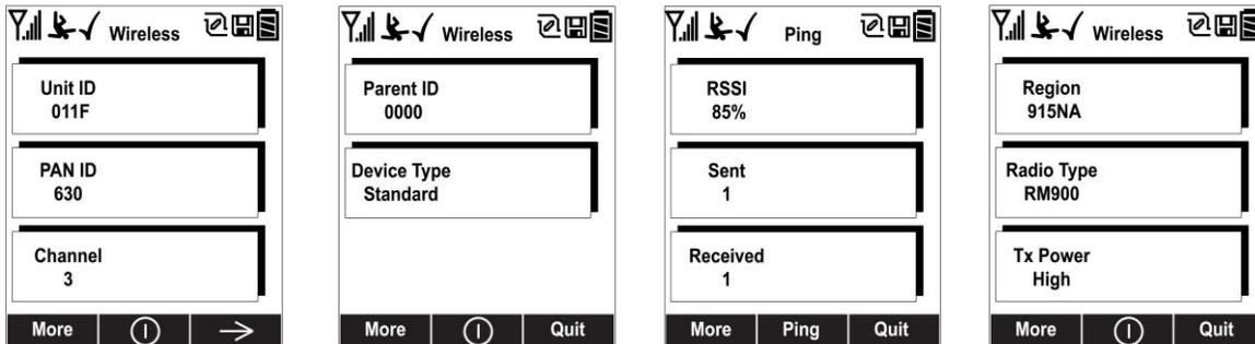
Unit ID (unique identifier of the instrument’s radio), Pan ID, and Channel are read-only parameters that help you to check whether the instrument’s wireless settings are correct (very helpful for troubleshooting).
