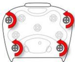
Remove the four screws holding the sensor compartment cover in place.
