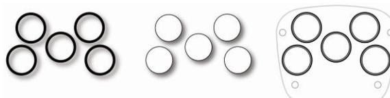
Remove the O-rings and then remove the filters. Replace them with new filters (press around the perimeter of each to ensure that the adhesive holds them firmly) and install the O-rings in their proper locations. O-rings may need to be replaced as well if they appear worn down, cracked, or dirty
