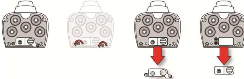
5. Press a new pump into place (a small amount of wiggling helps), making sure that both the inlet and outlet from the pump go into the two holes.
