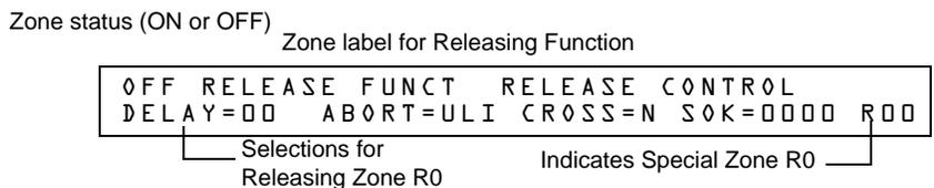
Figure 4.6 Sample Releasing Zone Read Status Display
