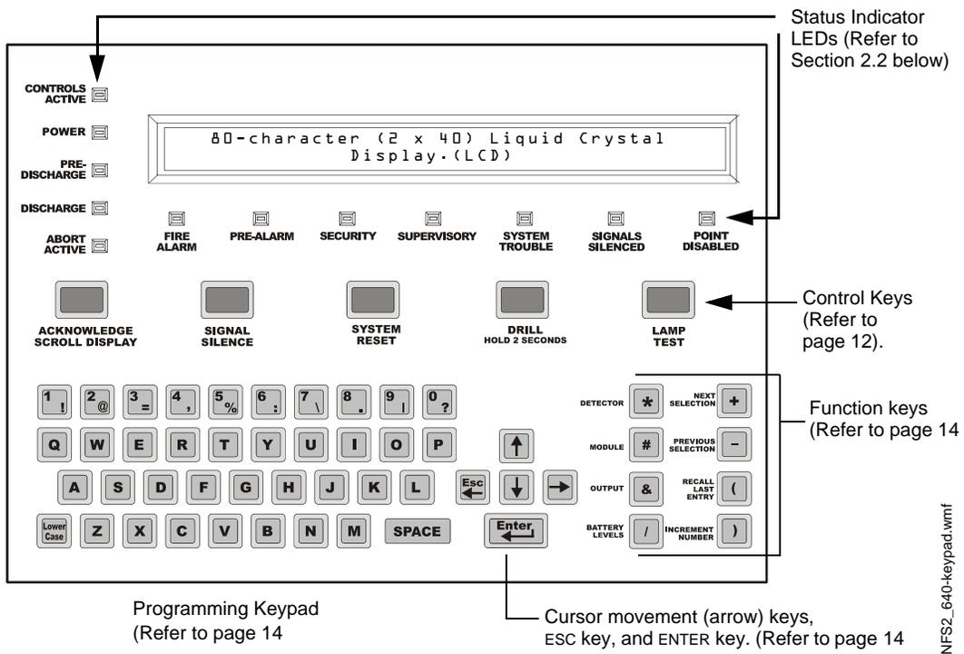
Figure 2.1 NFS-320 Control Panel Keys and Indicators
