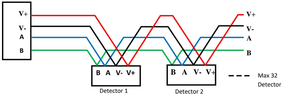
**Diagram 1: Panel to detector connections**
