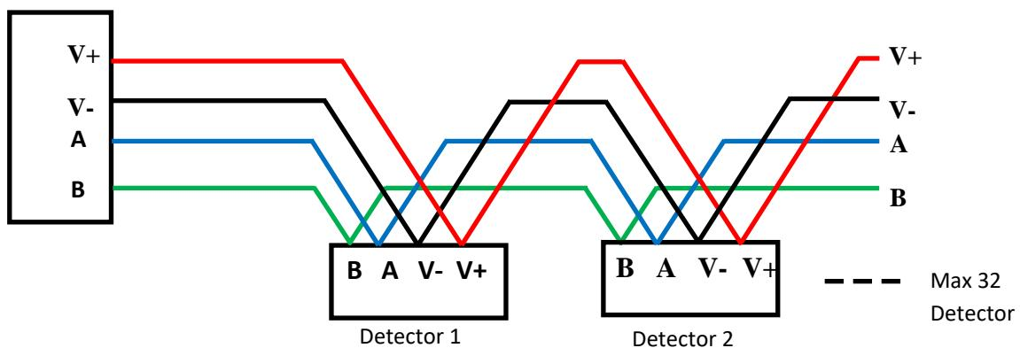
**Diagram 1: Panel to detector connections**
