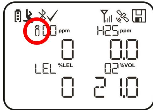
A bump test is required if the defined period of time between bump tests has been exceeded. This interval is set by an administrator using ProRAE Studio II.
