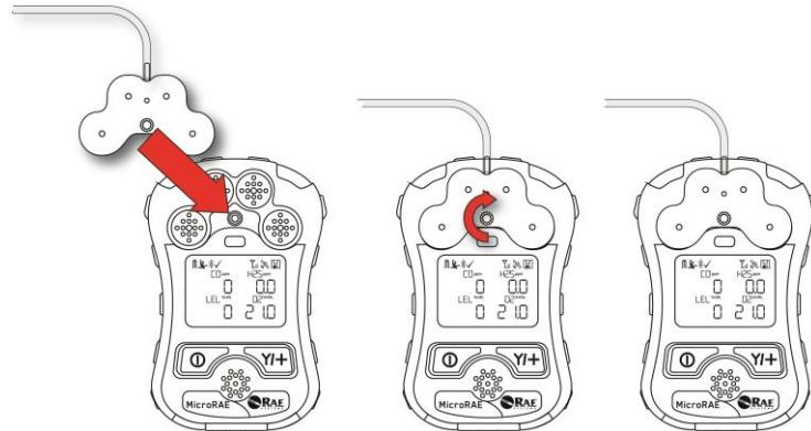
1. Align the Calibration Adapter's main body with the indented area around the MicroRAE's gas inlets.
