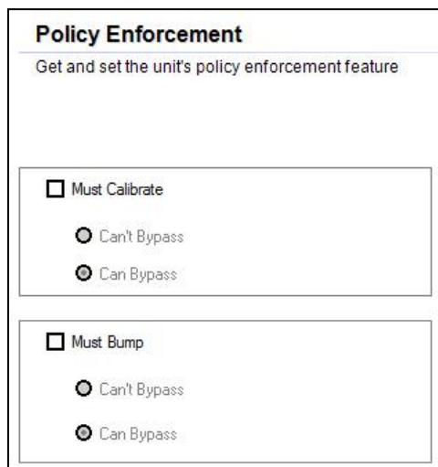
You can select “Must Calibrate” and/or “Must Bump” and then set whether the user must perform the selected operation in order to use the instrument.
