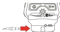
Plug the other end of the charger into a power source (AC outlet or mobile power port in a vehicle, depending on the model). When power is applied and the MicroRAE's battery is charging, the LED glows red. The LED glows green when the battery is fully charged.
