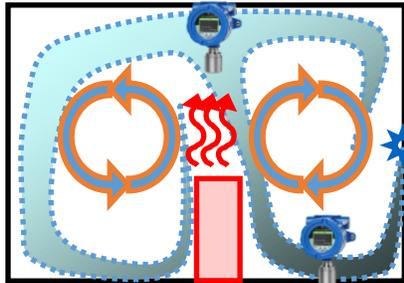
Vapor density of a gas determines if it will rise or fall in air when there are no significant currents. Lighter than air gases should have the detector mounted 12 to 18 inches (30 to 45 cm) above the potential gas leak, and heavier than air gases should be this distance below the potential gas leak.
