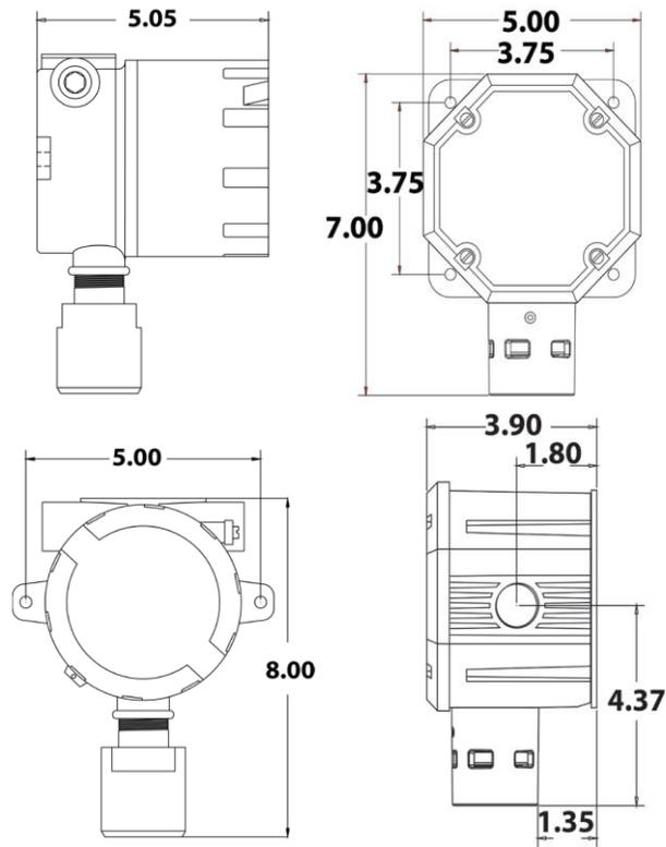
Figure 1 Mounting Dimensions
