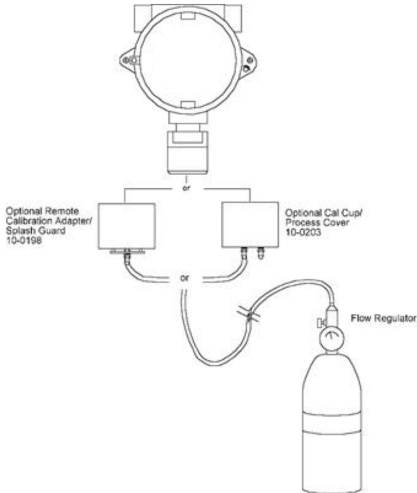
Figure 4 Calibration Diagram
