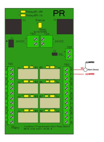
Figure 16 Programmable Relay Option Wiring Diagram
