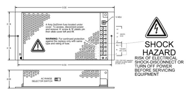
Figure 4 Optional 10-0172 150W 24VDC Power Supply Dimensions
