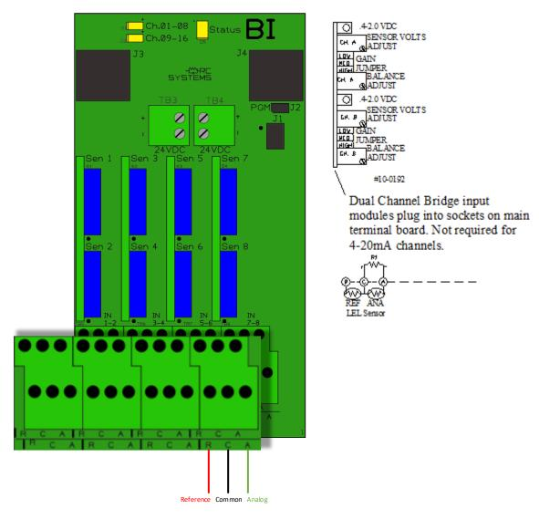
Figure 15 Bridge Input Wiring Diagram
