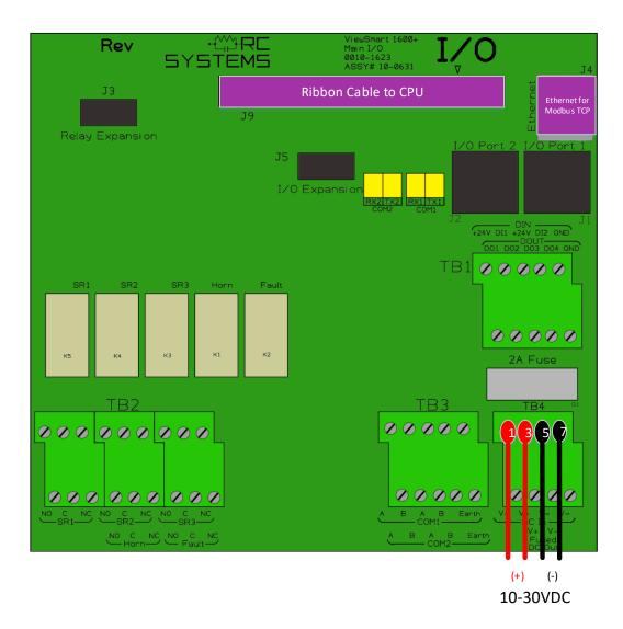
Figure 7 1600+ Main I/O Power Wiring Diagram
