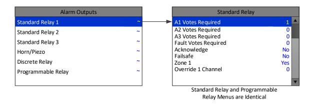
Figure 30 Standard Relay Configuration Menu
