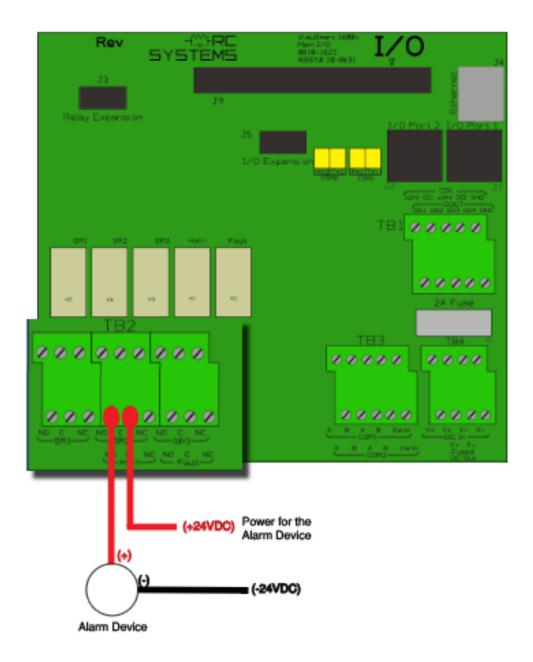
Figure 8 Common Relay Wiring
