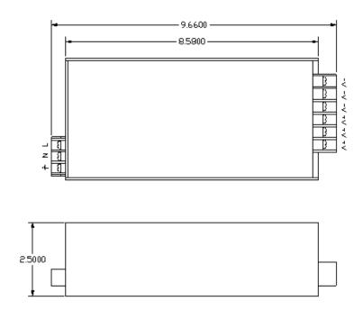
Figure 6 Optional 600W 24VDC Power Supply Dimensions
