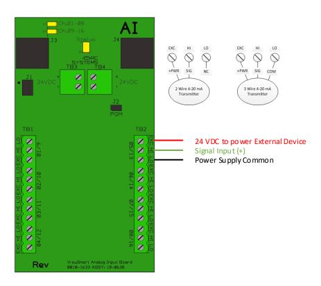
Figure 14 Analog Input Option Wiring Diagram
