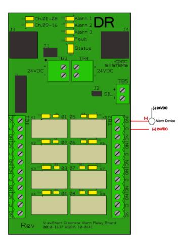
Figure 17 Discrete Relay Option Wiring Diagram
