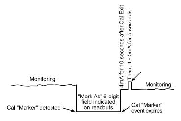
Figure 55 Sensor Life Transmission Diagram
