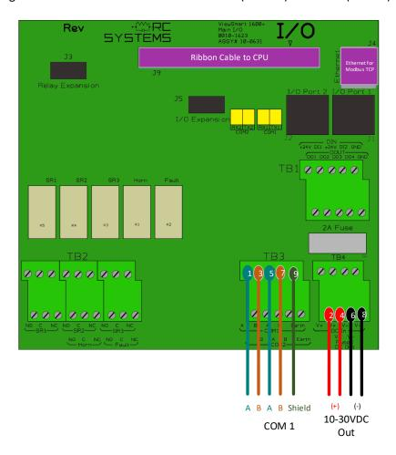
Figure 9 RS-485 Modbus® Wiring Diagram
