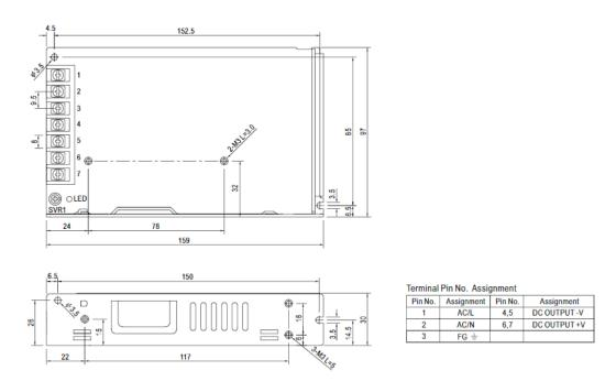
Figure 5 Optional 10-0673 150W 24VDC Power Supply Dimensions
