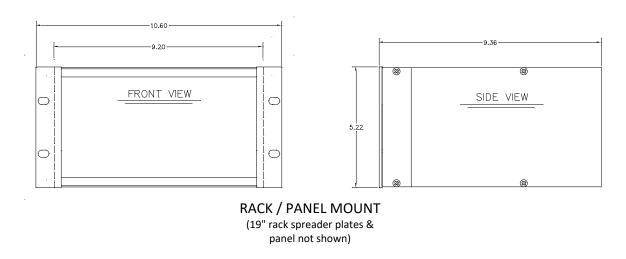
Figure 1 Panel/Rack Mount Dimensions
