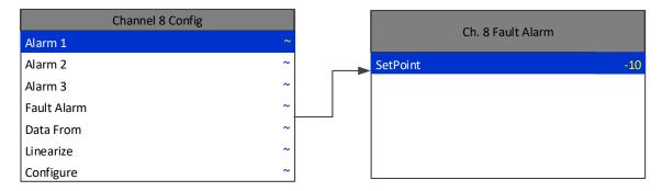
Figure 29 Fault Alarm Channel Config Menu
