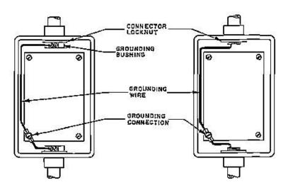
Figure 3 Grounding Instructions for Non-metallic Enclosures
