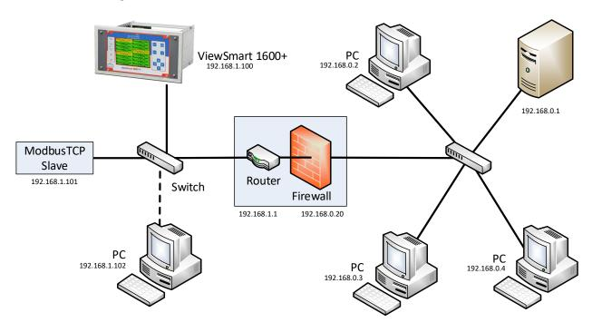
Figure 13 Modbus® TCP Connection over an Isolate Network
