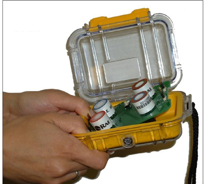
The standard alarm points and calibration values will automatically be loaded into the detector. Reassemble the detector and turn it on. Calibrate the EC sensor, and it is ready for use. **For the greatest safety and optimal performance, it is necessary to calibrate an EC sensor with its corresponding gas *anytime* it is moved from the SensorRAE to a detector.**
