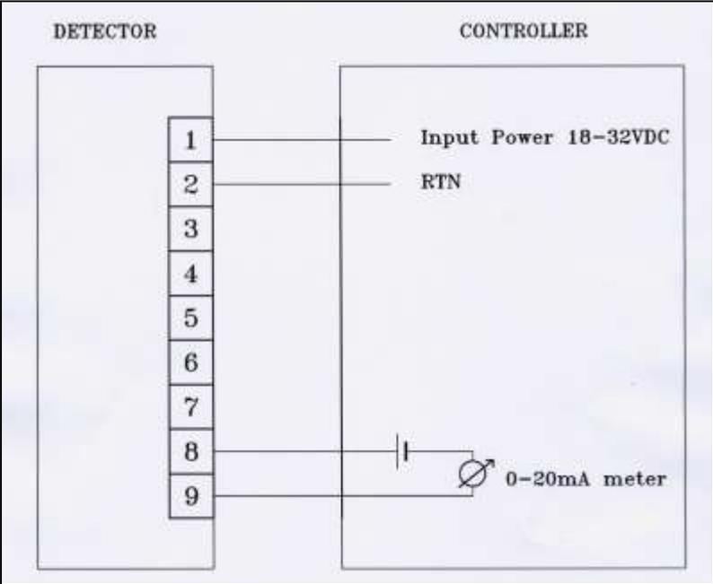
Figure 10: 0-20mA Wiring Option 1 (Sink 4-Wire) - Default
