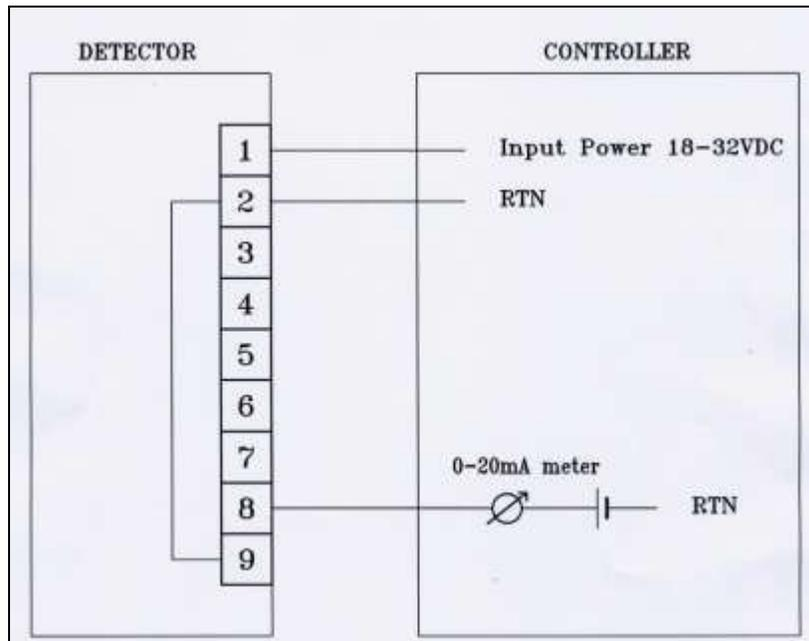
**Figure 12: 0-20mA Wiring Option 1 (Unisolated Sink 3-Wire)**
