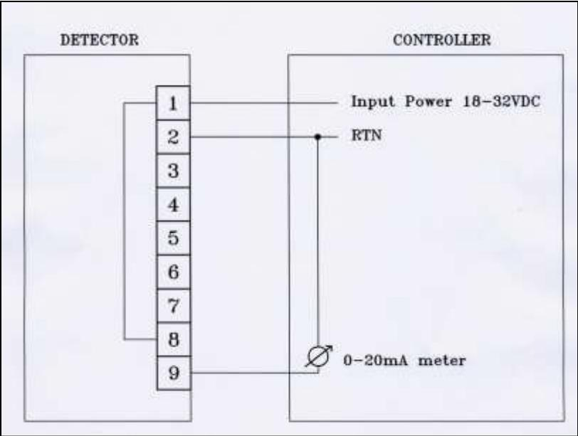
Figure 11: 0-20mA Wiring Option 1 (Converted to Source 3-Wire)
