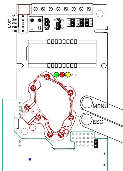
Figure 8. The ENTER command is done by pushing buttons MENU and ESC at the same time for about 14 seconds
