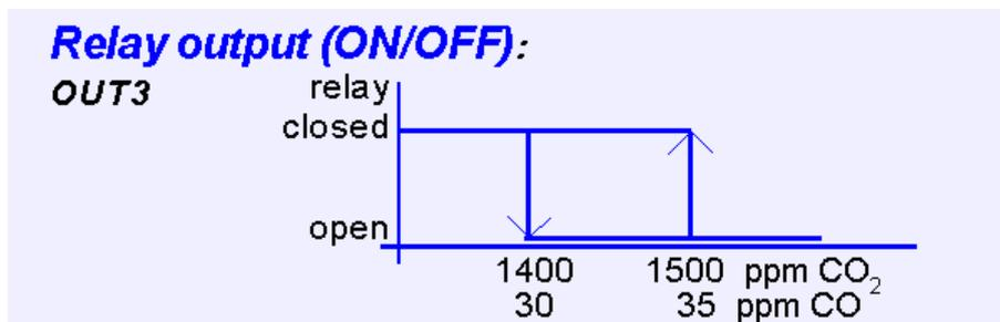
Figure 3. The control signal of air quality
