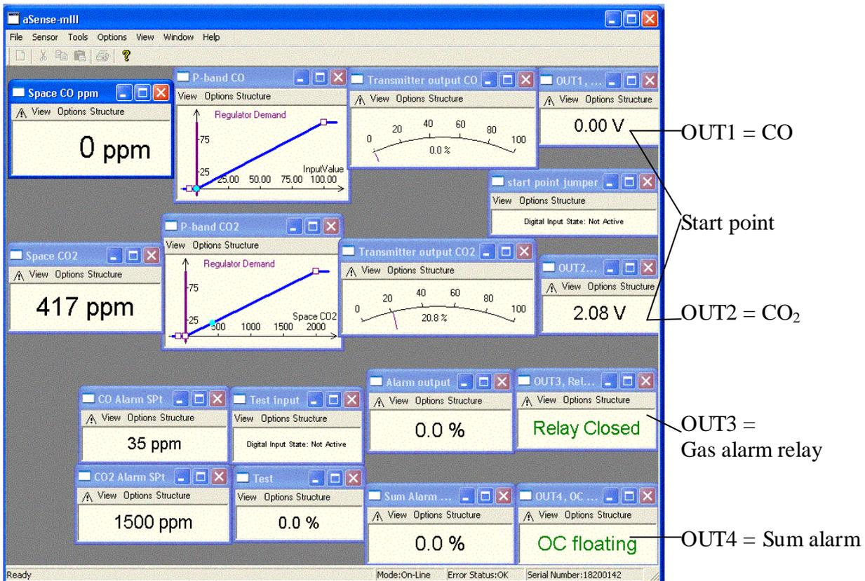
Figure 2. Print screen of *UIP4.3* PC work space of *aSENSE™ m III* where the pre set functions can easily be redefined. The four outputs (far right) are here arranged in rows together with the function blocks that controls the output
