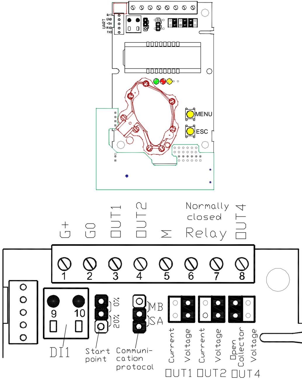
Figure 10. The *aSENSE™ m III* printed circuit board with the connection terminal area is enlarged. The terminal DI1 may be used for forced ventilation. If the sensor has a heater it is connected to G+ and G0.
