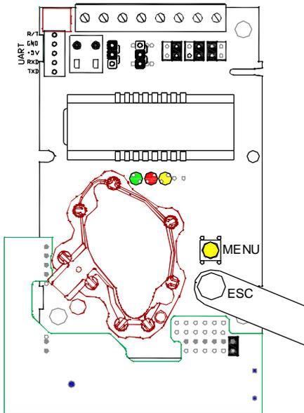
Figure 7. The push button MENU is pushed
