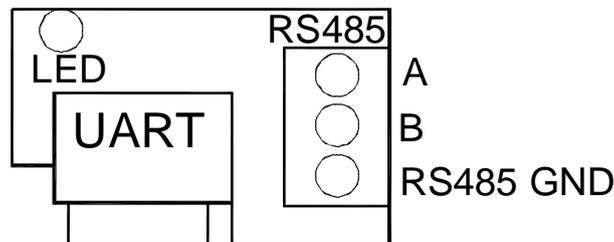
**The adapter is put on the UART connector with all five pins connected.** All five pins of the UART must be connected. The adapter should be mounted with the RS-485 terminal facing the other terminals and the LED facing the display.
