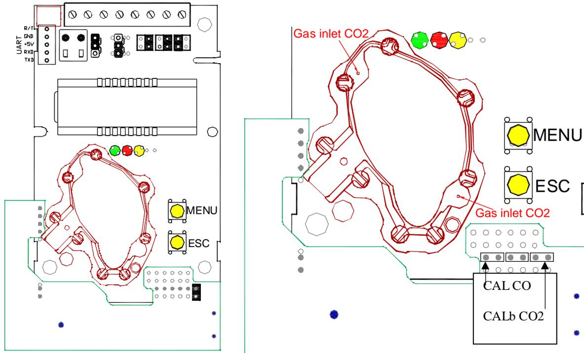
Figure 10. The PCB with the calibration jumper in default position. An enlarged part of the PCB with marked gas inlets and jumper positions for calibration is shown at right.
