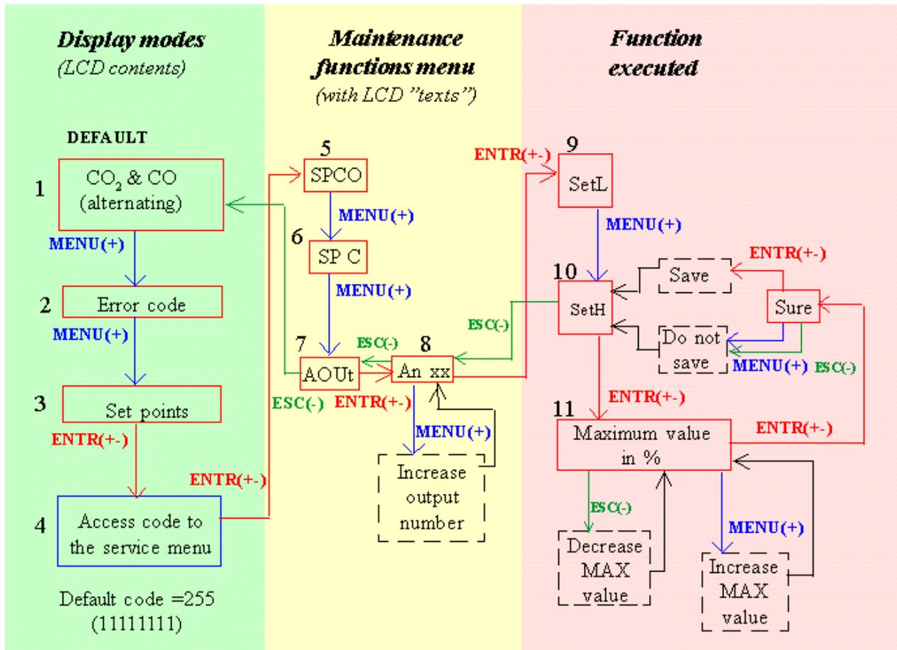
Figure 9. Maintenance functions available on *aSENSE™ m III* to set output limits. Only flow chart for setting High limits are shown, but Low limits are set in the very same way. The numbers in the flow chart refers to the points in example 1. Function blocks that are time limited are indicated by blue borders. Time limit refers to an internal time-out that returns the LCD and maintenance function back to normal. ENTER is a simultaneous pressing on MENU and ESC.
