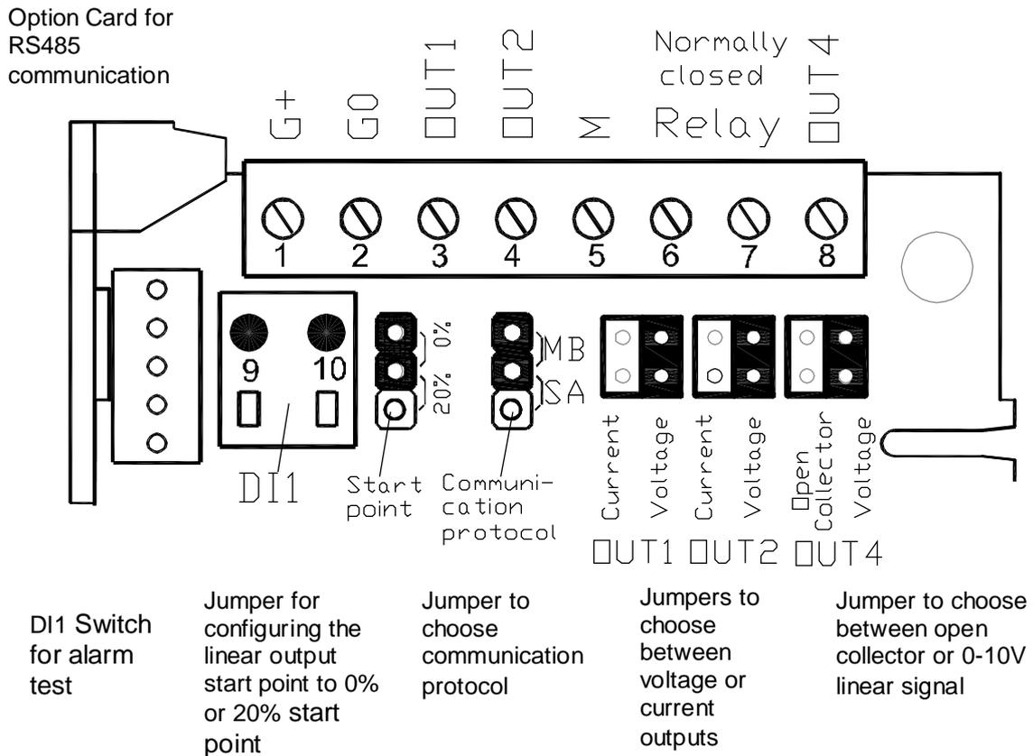
Figure 4. The connection terminal area of the *aSENSE™ m III* with jumpers and terminals. The terminal DI1 may be used for forced ventilation. If the sensor has a heater it is connected to G+ and G0.
