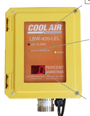
Alarm disabled indication. All relays will be deactivated when this LED is on.
