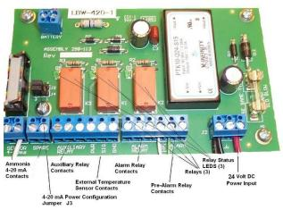
LBW-420-1 Enclosure Mounted Circuit Board
