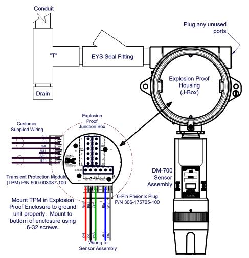
Figure 12 Typical Installation
