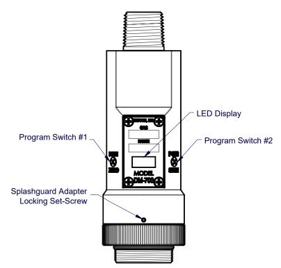
Figure 15 Magnetic Programming Switches
