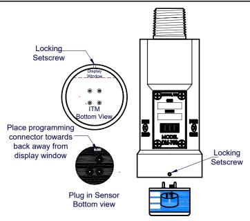
Figure 18 Sensor Cell and ITM Mating
