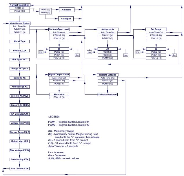
Figure 16 DM-700 Software Flowchart
