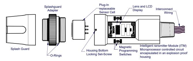
Figure 17 Sensor Assembly
