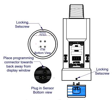
Figure 19 Sensor Cell and ITM Mating
