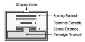
Figure 1 Construction of Electrochemical Toxic Sensor
