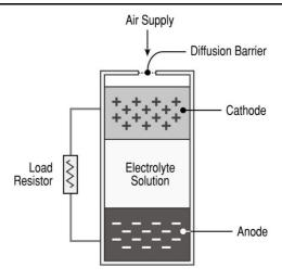
Figure 2 Construction of Galvanic Cell
