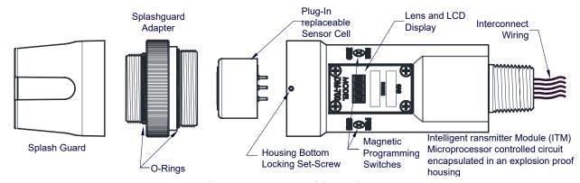
Figure 5 Sensor Assembly Breakaway
