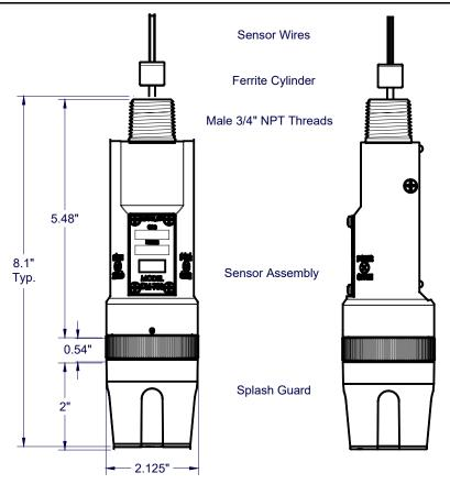
Figure 8 Outline and Mounting Dimensions (Sensor Assembly only)
