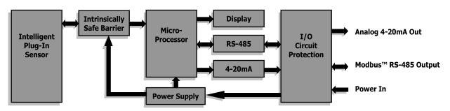
Figure 3 ITM Circuit Functional Block Diagram
