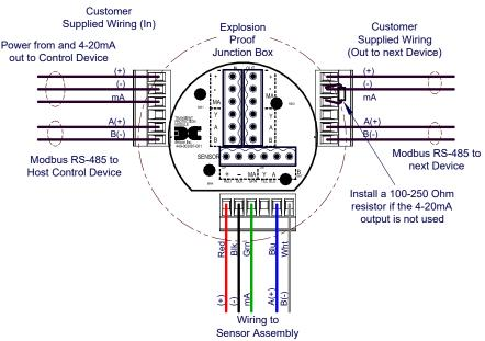
Figure 13 Sensor Wire Connections
