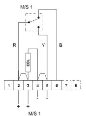
1A - Circuit shown in Unoperated condition (Glass Intact)
