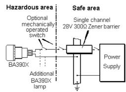
Fig 1 Typical BA390X lamp circuit
