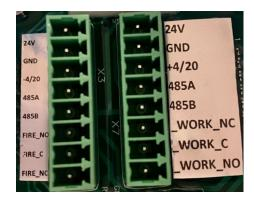
Figure 5-2: Arrangement and Functions of Mounting Connection Terminals
