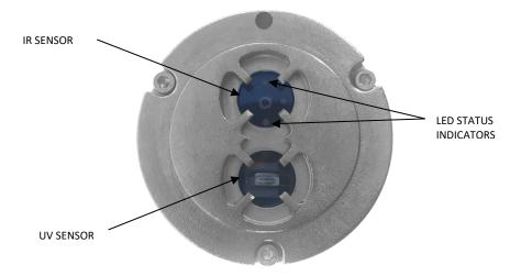
Figure 4-2: IR & UV Detectors and LED Indicators
