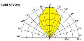
To meet the requirements of EN54:10 clause 5.4, where the ratio of the response points Dmax: Dmin should not exceed 1.41, the horizontal and vertical viewing angles max should not exceed  $\pm 30^\circ$ .
