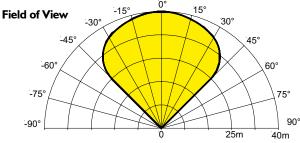
To meet the requirements of EN54:10 clause 5.4, where the ratio of the response points Dmax: Dmin should not exceed 1.41, the horizontal and vertical viewing angles max should not exceed  $\pm 20^{\circ}$
