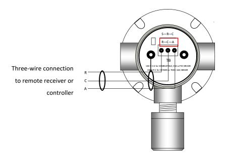
Figure 4-2: GDS-48 Wiring Connections (Gray Enclosure)
