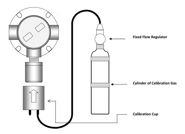
Figure 5-1: Applying Calibration Gas to GDS-48
