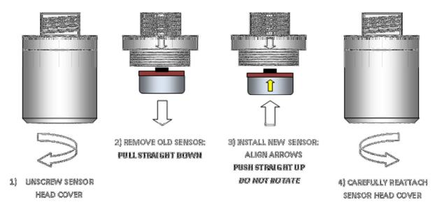
Figure 6-1: Sensor Replacement
