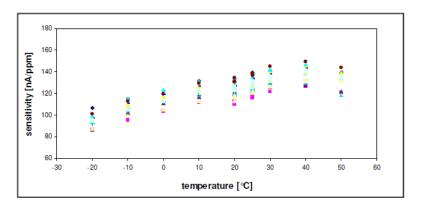
knowledge of the sensor's actual temperature. The GASMAX CX gas sensor used in the GDS-68SXP provides this temperature compensation.
