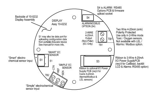
FIGURE 1: TRANSMAX / EC DISPLAY BOARD
