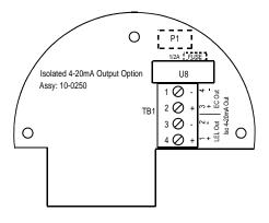
FIGURE 5: TRANSMAX II Isolated 4-20mA Output Board
