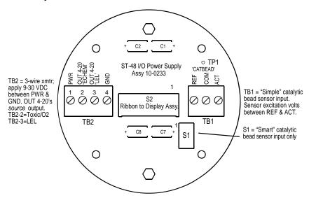
FIGURE 2: TRANSMAX II I/O Power Supply Board
