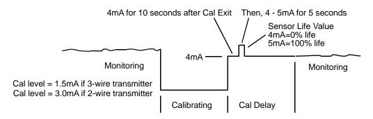
Figure 8: Transmit Sensor Life Timing Diagram
