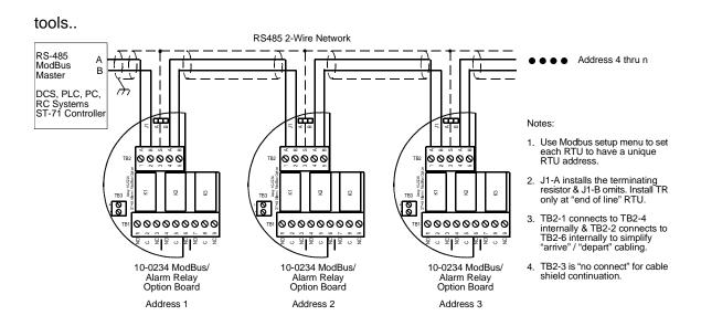
FIGURE 4: TRANSMAX II Alarm / MODBUS Board
