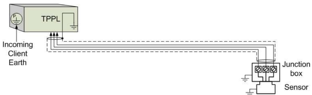
Figure 32. Grounding for Screened Cable, No Armour, with Metal Junction Box and Sensor
