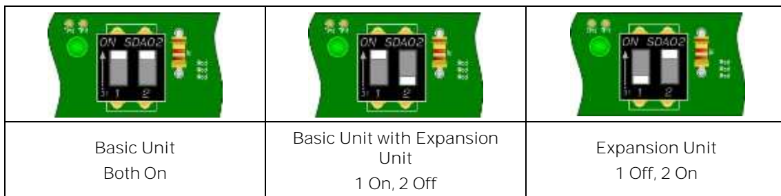
Figure 12. Backplane DIP Switch Settings
