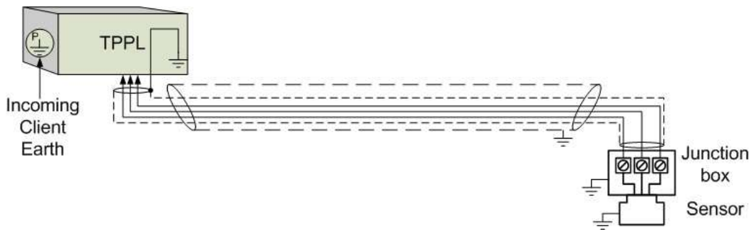
Figure 31. Grounding for Screened Cable with Armour and with Metal Junction Box and Sensor
