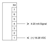
LC-1112 (0)4-20 mA signal, 3-wire, 24 VDC
