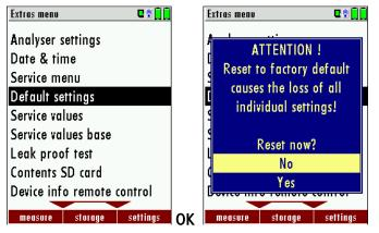
The analyzer will be reset to original delivery settings.
