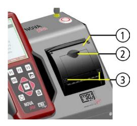
To change the printer paper you pull out the little plastic recessed grip (2) which is mounted on the transparent printer cover (1). Insert the new printer roll and let the end of the paper stick out of the printer (+/- half inch). Close the printer cover (marking 3) using only with light pressure. Paper feed is activated using the printer button (when not in measuring window).
