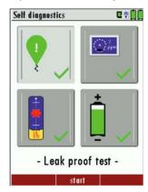
Top left: Leak proof test Top right: sensor test Bottom left: flow control Bottom right: Battery status
