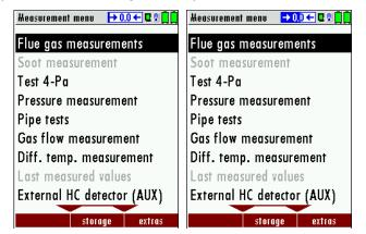
The unit will display a self-test after zeroing (Leak tight test, sensor test, internal flow monitoring and battery status). The unit will display any error (for example defect sensor) that is detected during the self-test. With the ESC button you can delete any displayed error messages and then reach the measuring menu.
