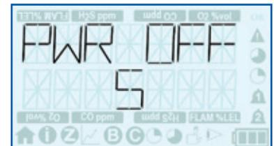
The **MG-1** cannot be shutdown if a zero, bump test or calibration is in progress.
