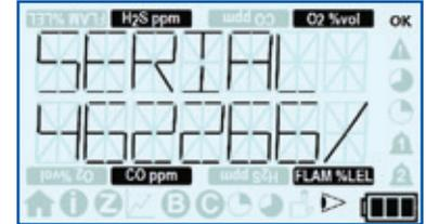
The screen then displays the **MG-1** firmware version.
