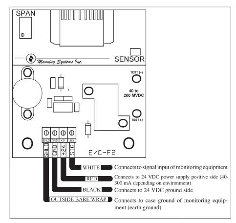
Figure 2: Wiring diagram for the EC-F2 Sensor
