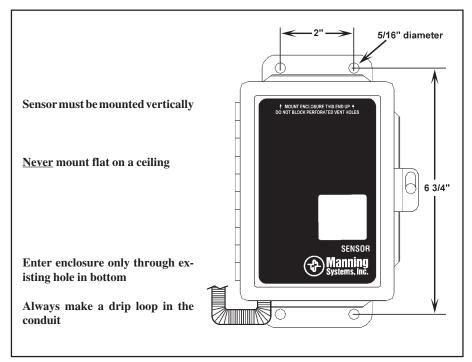
Figure 1: Mounting dimensions for the EC-F2 Sensor
