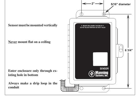
Figure 1: Mounting dimensions for the EC-F2 Sensor
