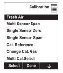
After a timer countdown, the zero calibration is done. The LCD displays the sensor names and tells you whether each calibration passed or failed, followed by the sensor readings.
