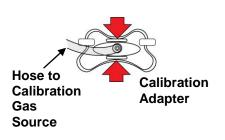
Grasp the small handles on the Calibration Adapter.
