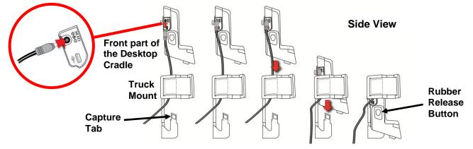
Place the MultiRAE into the cradle (make sure the bottom of the instrument and the alignment pins on the cradle mate properly) and press down until it is locked in place. Then wrap the Velcro strap around the MultiRAE and fasten its end to the mating Velcro on the side of the Truck-Mount.
