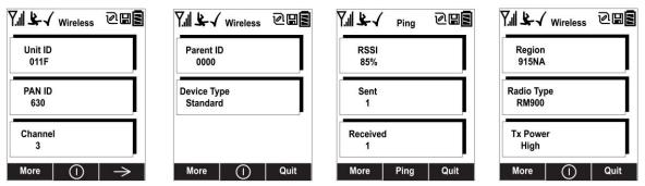
Unit ID (unique identifier of the instrument's radio), Pan ID, and Channel are read-only parameters that help you to check whether the instrument's wireless settings are correct (very helpful for troubleshooting).
