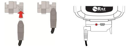
Plug the other end of the charger into a power source (AC outlet or 12VDC mobile power port, depending on the model). When power is applied and the MultiRAE's battery is charging, the LED glows red. The LED glows green when the battery is fully charged.
