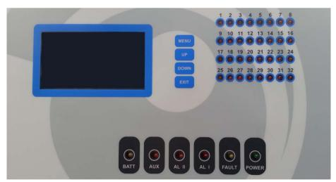
Diagram 8: Front panel signs LCD and LEDs
