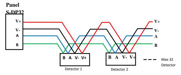
**Diagram 13: Panel to detector connections**
