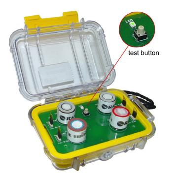
The standard alarm points and calibration values will automatically be loaded into the detector. Reassemble the detector and turn it on. Calibrate the EC sensor, and it is ready for use. For the greatest safety and optimal performance, it is necessary to calibrate an EC sensor with its corresponding gas *anytime* it is moved from the SensorRAE to a detector.
