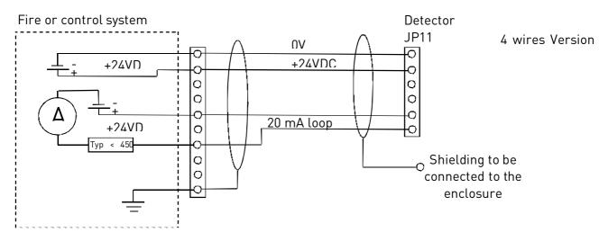
When using a 4 wires connection, the current loop is provided by the input module or PLC. The loop (L + and L-) is optically isolated from the detector. 4-20mA or 0-22mA input module of the PLC has to power up the current loop with, at least 8V at the terminal level, for 22 mA. This reduces the resistance of the loop as defined in the relationship below.
