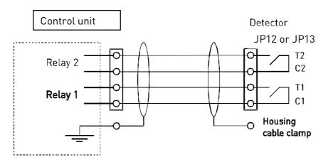
The two relays can be configured normally closed or normally open. If normally open, the relays are opened when they are not powered (power loss).
