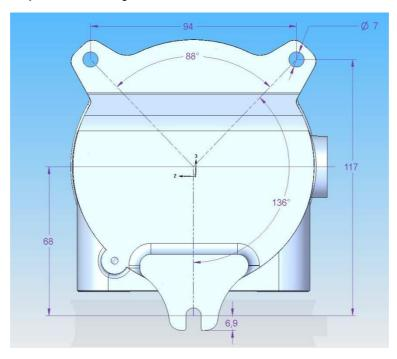
Figure 3 : Drilling dimensions for support fixing.
