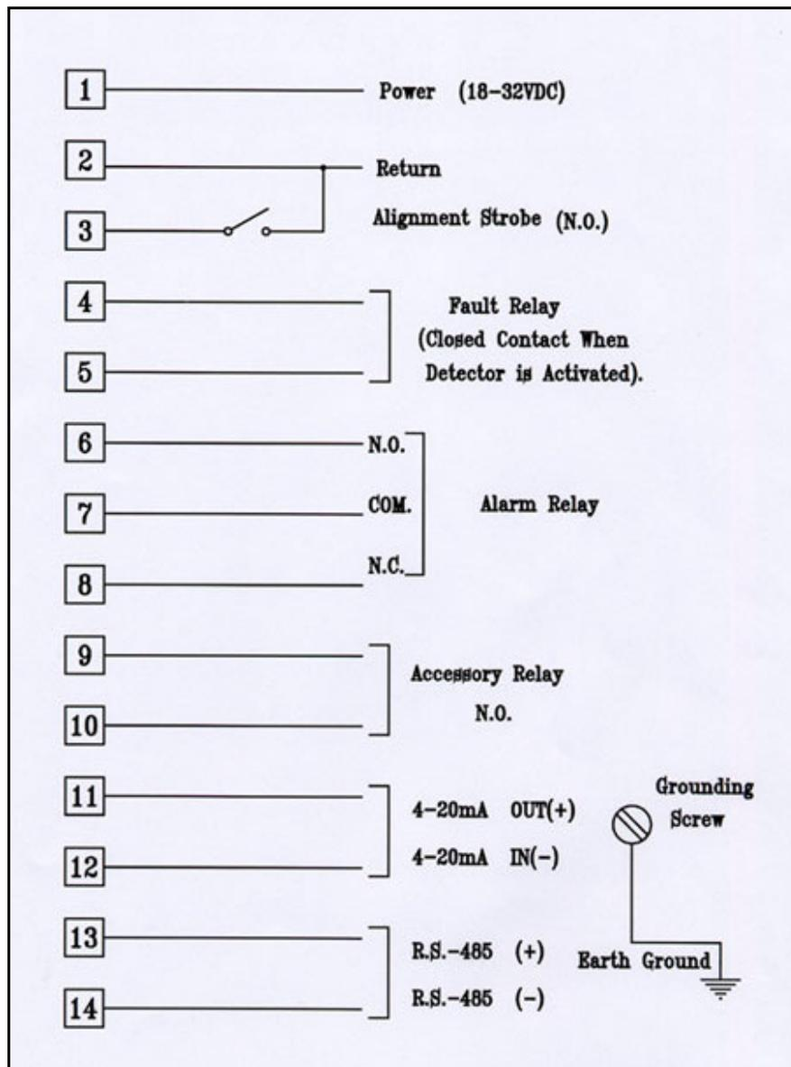
Figure 3. Detector's Wiring Diagram
