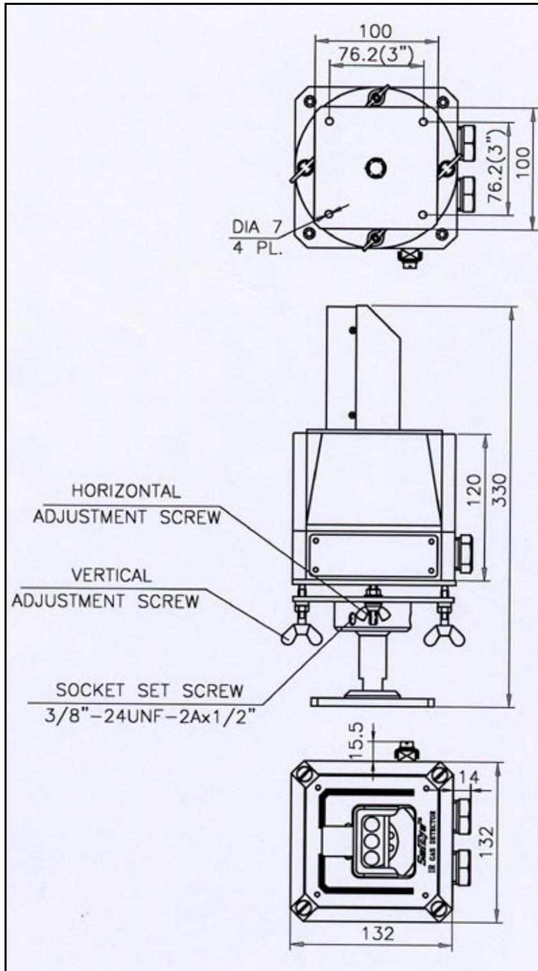
Figure 21. Detector Outline Drawing With Swivel Mount
