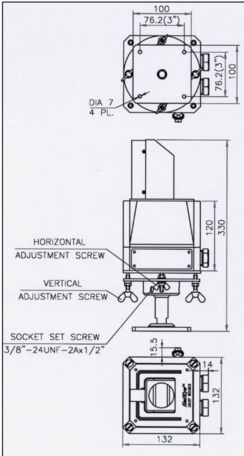
Figure 22. Source Outline Drawing (Reflector Type) With Swivel Mount
